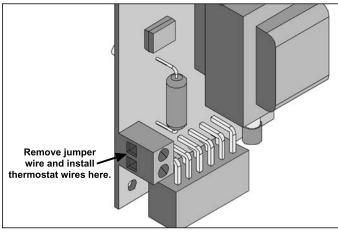
Figure 21: Thermostat wire placement.
